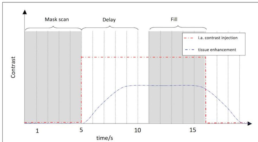
Figure 1. Injection and acquisition protocol for C-arm CT blood volume measurements.
