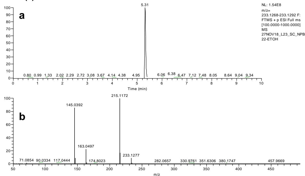
**S2.7 5F-PB-22 ester hydrolysis detection/confirmation: full scan MS EIC (a) and MS<sup>2</sup> at NCE 20 (b)**
