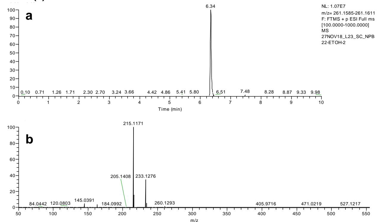
**S2.3 5F-PB-22 ethyl ester detection/confirmation: full scan MS EIC (a) and MS<sup>2</sup> at NCE 30 (b)**
