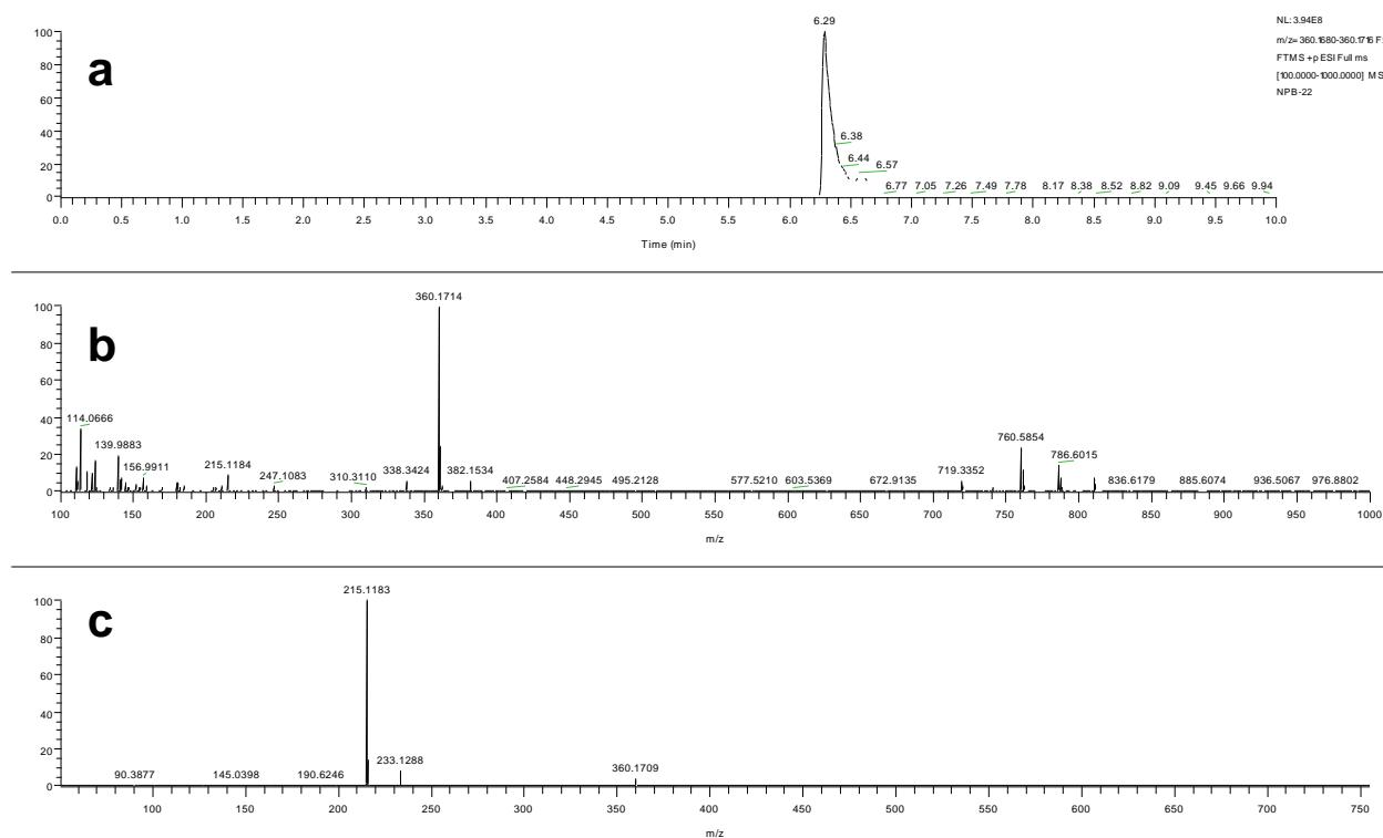
**S1.26 LC-HRMS (a), full scan MS spectrum (b) and MS<sup>2</sup> at NCE 13 (c) of 5F-PB-22**
