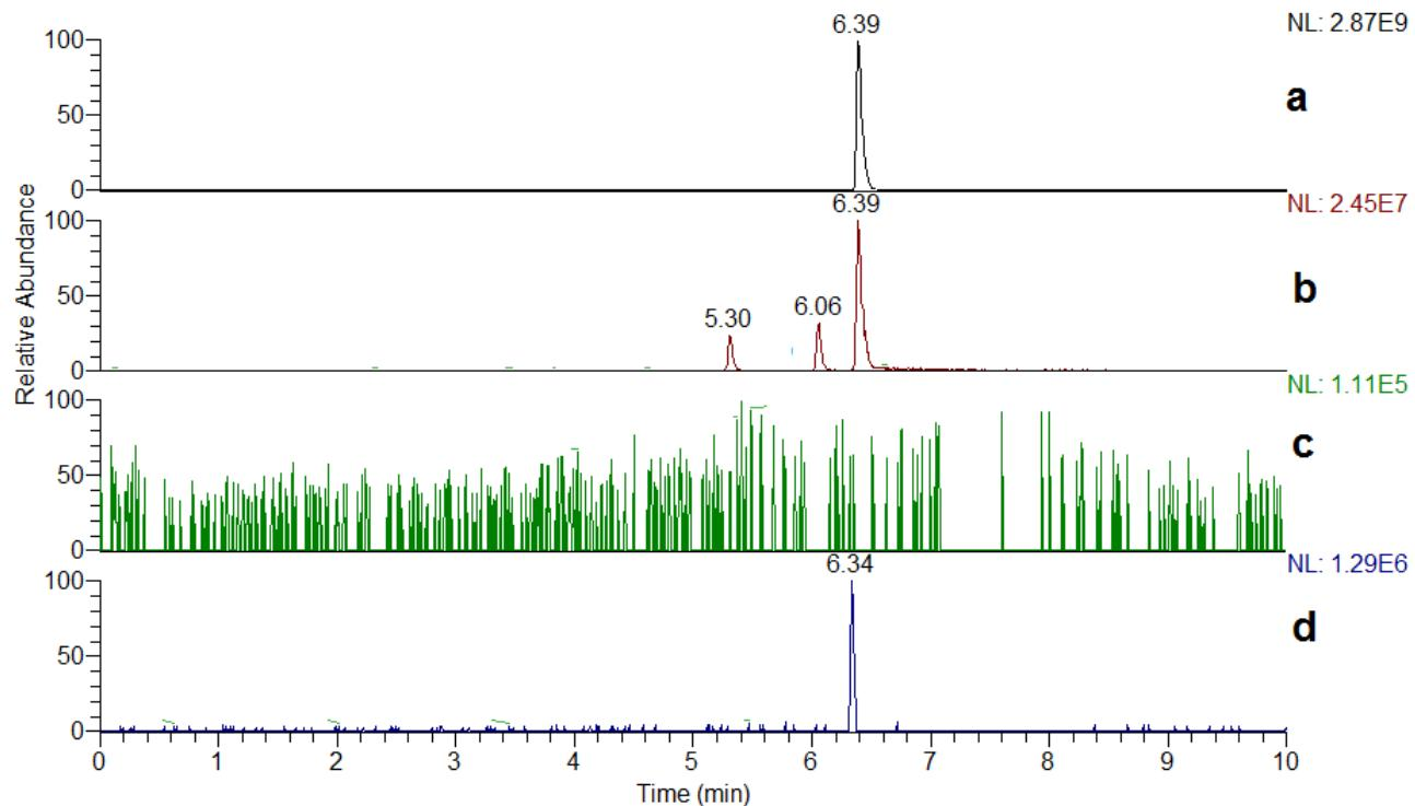
Overlaid extracted ion chromatograms (exact mass  $\pm$  2.5 ppm) of the major detected 5F-NPB-22 HLM-derived metabolites (S3.12-S3.14) in the presence of ethanol, ethanol + inhibitor and negative control: a = parent drug 5F-NPB-22; b = ester hydrolysis (**12**); c = ester hydrolysis plus monohydroxylation; d = ester hydrolysis plus oxidative defluorination ; e = 5F-NPB-22 ethyl ester (**10**)
