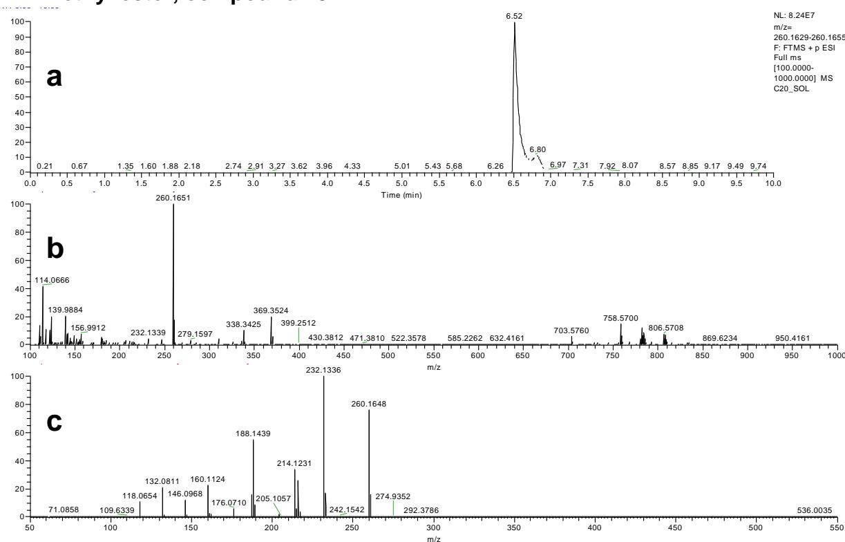
**S1.29 LC-HRMS (a), full scan MS spectrum (b) and MS<sup>2</sup> at NCE 30 (c) of synthesised NPB-22 ethyl ester, compound 11**
