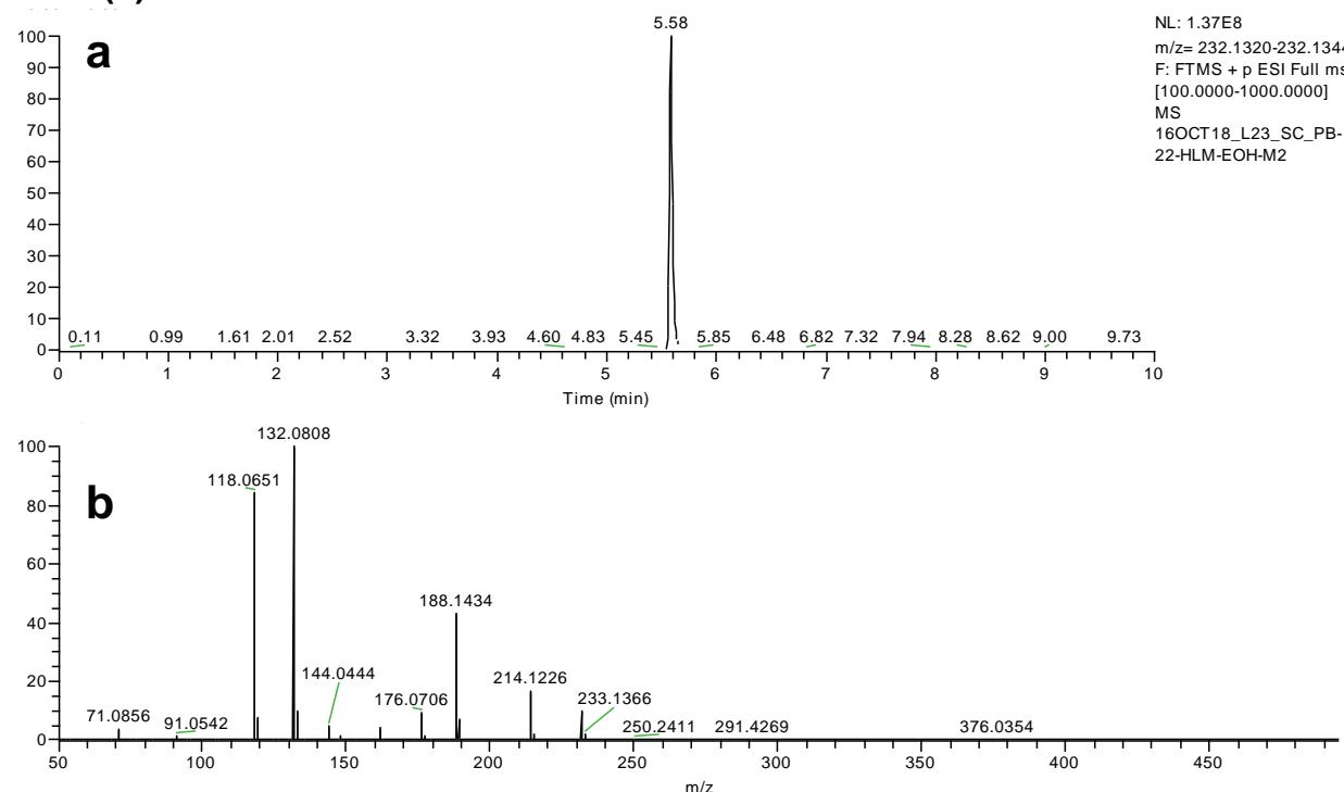
**S2.6 NPB-22 ester hydrolysis detection/confirmation: full scan MS EIC (a) and MS<sup>2</sup> at NCE 45 (b)**
