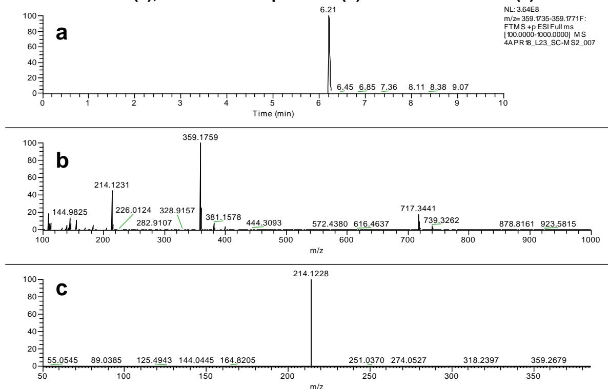
**S1.25 LC-HRMS (a), full scan MS spectrum (b) and MS<sup>2</sup> at NCE 20 (c) of NPB-22**
