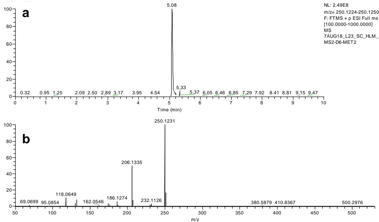
**S2.8 5F-NPB-22 ester hydrolysis detection/confirmation: full scan MS EIC (a) and MS<sup>2</sup> at NCE 45 (b)**
