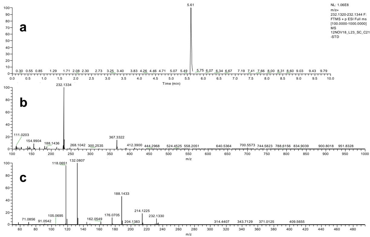
**S1.33 LC-HRMS (a), full scan MS spectrum (b) and MS<sup>2</sup> at NCE 45 (c) of synthesised NPB-22-COOH, compound 13**
