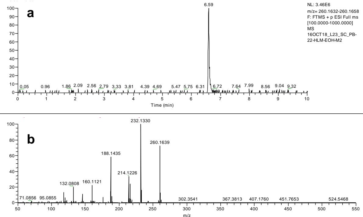
**S2.2 NPB-22 ethyl ester detection/confirmation: full scan MS EIC (a) and MS<sup>2</sup> at NCE 30 (b)**
