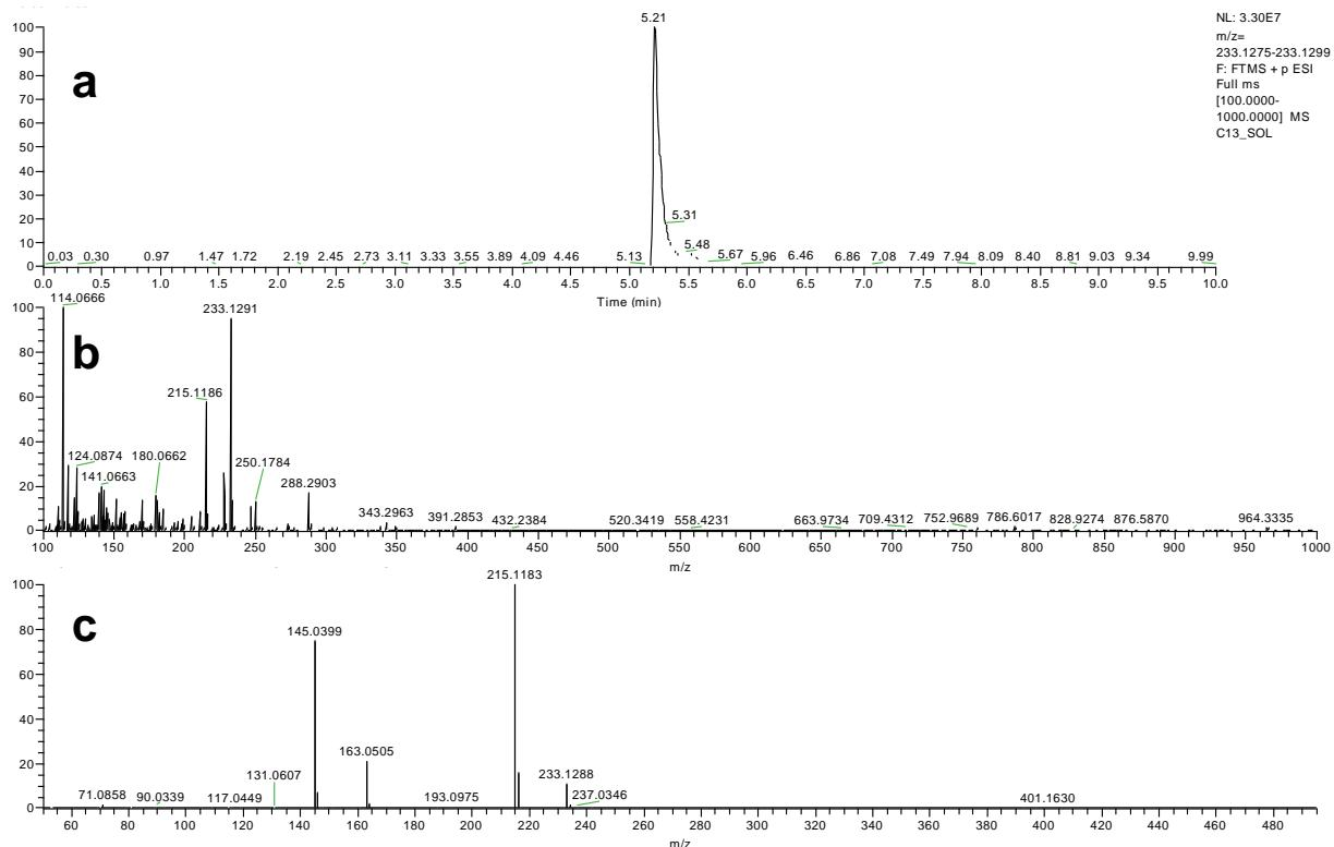
**S1.34 LC-HRMS (a), full scan MS spectrum (b) and MS<sup>2</sup> at NCE 20 (c) of synthesised 5F-PB-22-COOH, compound 16**
