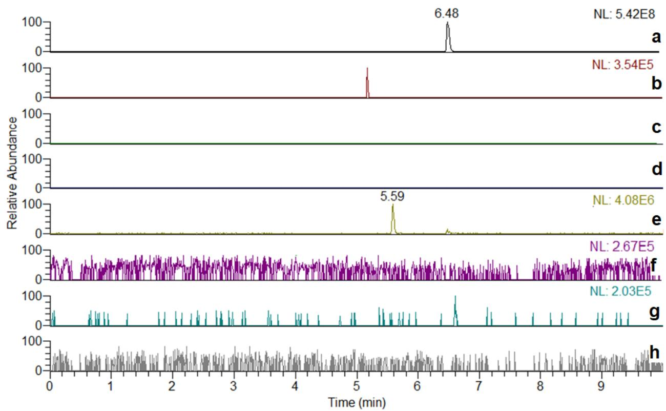
Overlaid extracted ion chromatograms (exact mass  $\pm$  2.5 ppm) of the major detected 5F-PB-22 HLM-derived metabolites (**S3.5-S3.8**) in the presence of ethanol, ethanol + inhibitor and negative control: a = parent drug 5F-PB-22; b = monohydroxylation; c = carbonylation; d = monohydroxylation plus N-dealkylation; e = ester hydrolysis (**16**); f = ester hydrolysis plus monohydroxylation; g = 5F-PB-22 ethyl ester (**14**); h = 5F-PB-22 ethyl ester plus monohydroxylation
