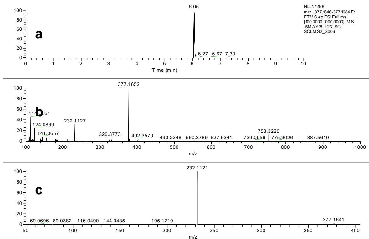
**S1.27 LC-HRMS (a), full scan MS spectrum (b) and MS<sup>2</sup> at NCE 20 (c) of 5F-NPB-22**
