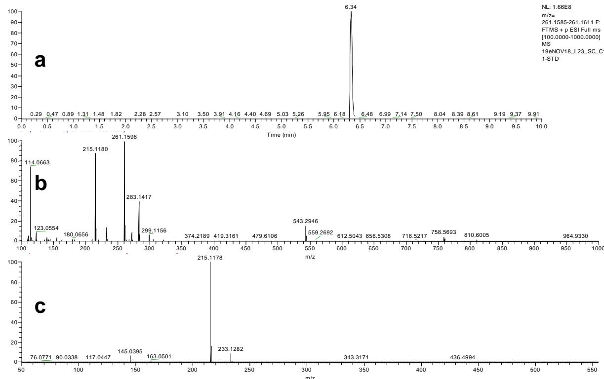
**S1.30 LC-HRMS (a), full scan MS spectrum (b) and  $\text{MS}^2$  at NCE 30 (c) of synthesised 5F-PB-22 ethyl ester, compound 14**
