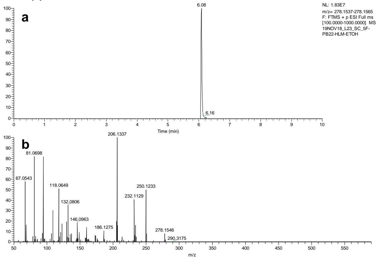
**S2.4 5F-NPB-22 ethyl ester detection/confirmation: full scan MS EIC (a) and MS<sup>2</sup> at NCE 35 (b)**
