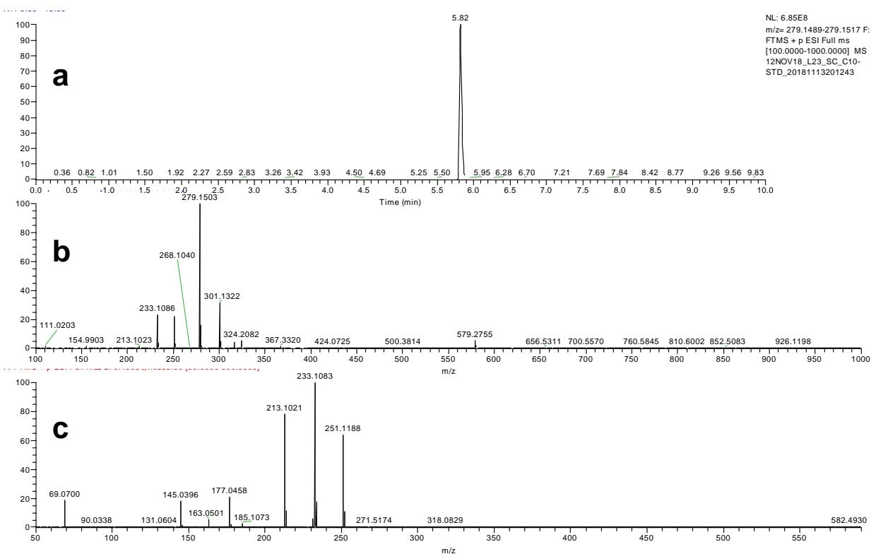
**S1.32 LC-HRMS (a), full scan MS spectrum (b) and MS<sup>2</sup> at NCE 40 (c) of synthesised PB-22 COOH, compound 17**
