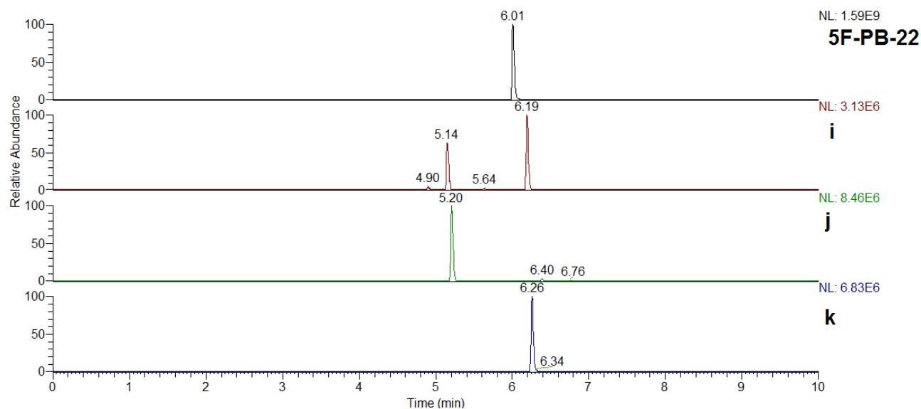
Overlaid extracted ion chromatograms (exact mass  $\pm$  2.5 ppm) of the major detected NPB-22 HLM-derived metabolites (S3.9-S3.11) in the presence of ethanol, ethanol + inhibitor and negative control: a = parent drug NPB-22; b = ester hydrolysis (**13**); c = ester hydrolysis plus monohydroxylation; d = NPB-22 ethyl ester (**11**)
