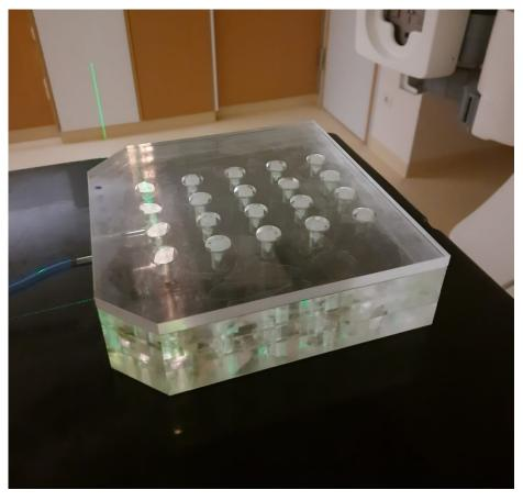
Supplementary figure 3 Plexiglass sample holder used for photon irradiation The 1.5 ml Eppendorf tubes with samples were placed in drill holes in the plexiglass block and covered with a plexiglass top.
