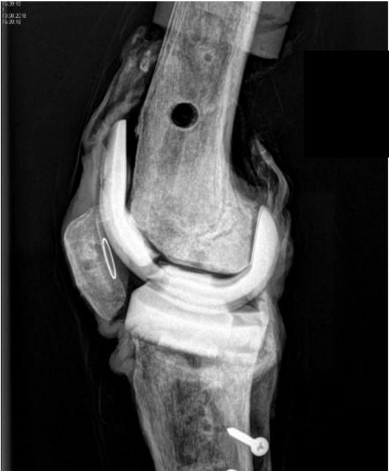
Figure S2: Broken femoral component of COPAL knee spacer of one specimen during cyclic loading to 2600 N
