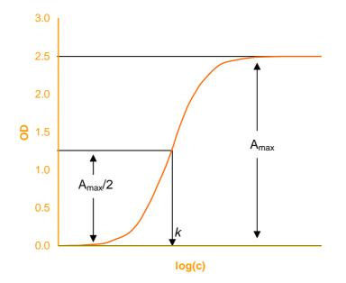
The concentration, s, of any sample, in terms of the standard, can now be read off this curve or estimated using the rearranged relationship :
