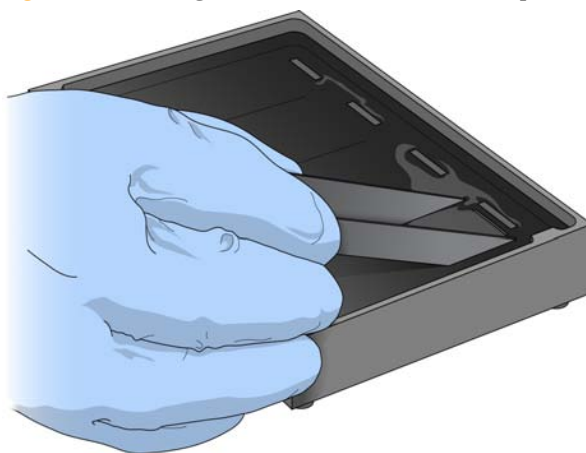
Figure 120 Placing Black Frames into Multi-Sample BeadChip Alignment Fixture
