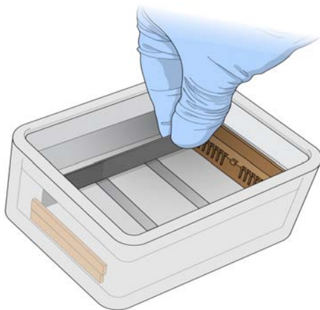
Figure 119 Submerging BeadChips in Wash Dish Containing PB1
