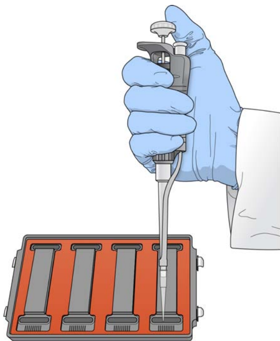
Figure 33 Dispensing PB2 into Hyb Chamber Reservoir
