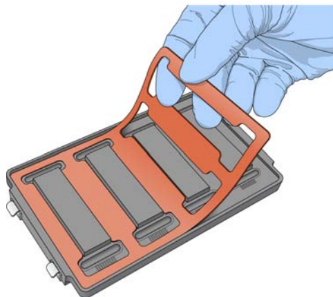
Figure 102 Placing Gasket into Hyb Chamber
