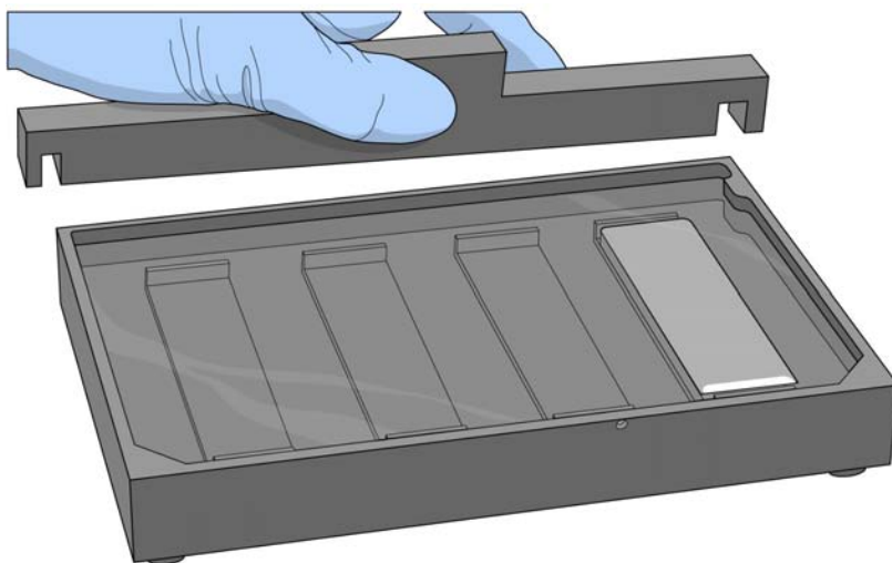
Figure 123 Placing Alignment Bar onto Alignment Fixture
