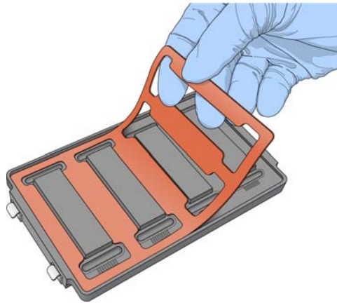
Figure 31 Placing Gasket into Hyb Chamber
