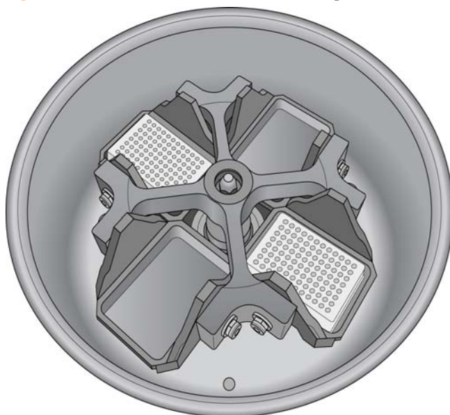
Figure 25 Sealed MSA4 Plate and Plate of Equal Balance in Centrifuge
