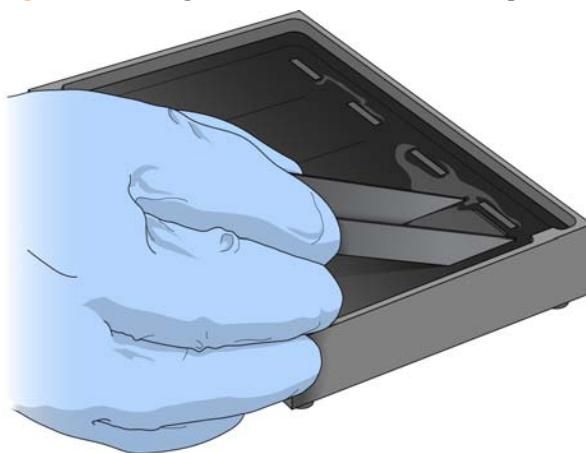
Figure 51 Placing Black Frames into Multi-Sample BeadChip Alignment Fixture
