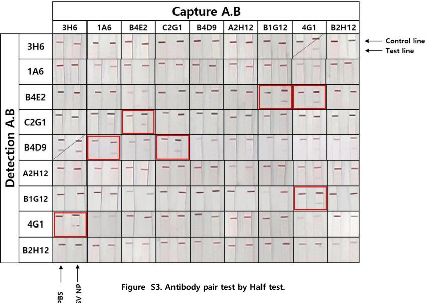
Half strip test was performed with all 81 capture-detection combinations for produced 9 SFTSV N antibodies. It was carried out by the lateral flow immunoassay (LFIA) method without sample pad and conjugated pad. The test strip was coated with each of 9 SFTSV N antibodies as capture antibody, and dipped in the mixture of SFTSV N protein (100ng/ml) as antigen and each 9 antibodies as detection antibodies.
