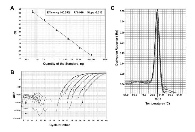
Optimization of Real-Time PCR conditions. (A) SEMA3C standard curve consisted of 6 points of the reference sample (reference human brain RNA), 5x dilutions (150, 30, 6, 1.2, 0.24, 0.048 ng/well). All dilution points were done in 3 replicates. SEMA3C standard curve parameters: efficiency 100.2 %, R2 0.99, slope -3.31, thereby confirming the suitability of PCR conditions and primers for mRNA quantitation. (B) Amplification plot. (C) Melting curve analysis of PCR products.
