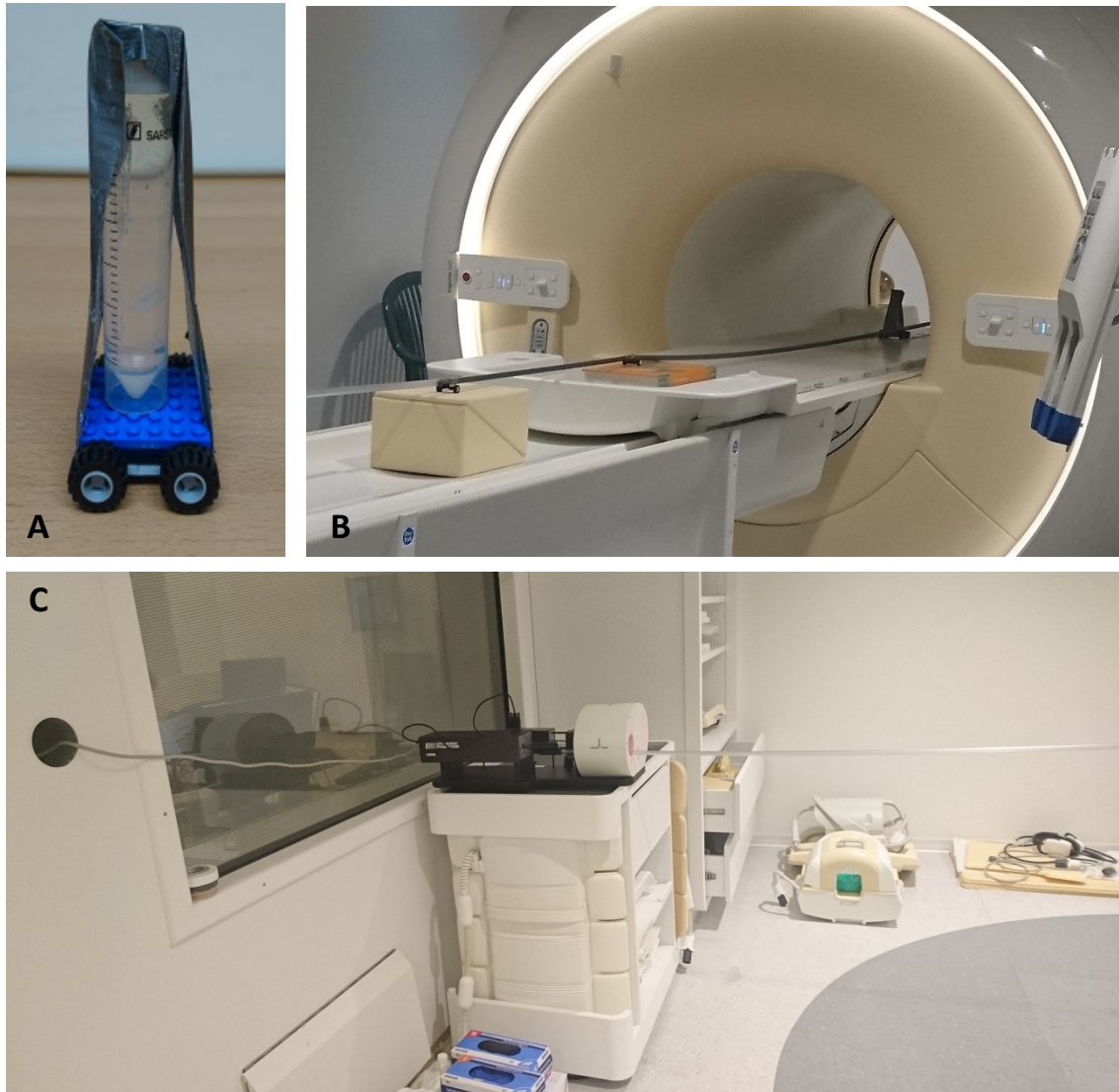
Figure S2: Phantom study set-up. (A) MR compatible phantom consisting of a tube, filled with 1% \text{CuSO}_4 aqueous solution, fixed onto a Lego cart. (B) The phantom in the scanner bore, connected to the motion translating extension. Extension rods are supported to avoid slack from generator to phantom. To reduce friction between extension rods and supporting elements, they are guided via Lego wheels. (C) CIRS Dynamic Thorax Phantom; motion generator with extension for motion translation to the phantom.
