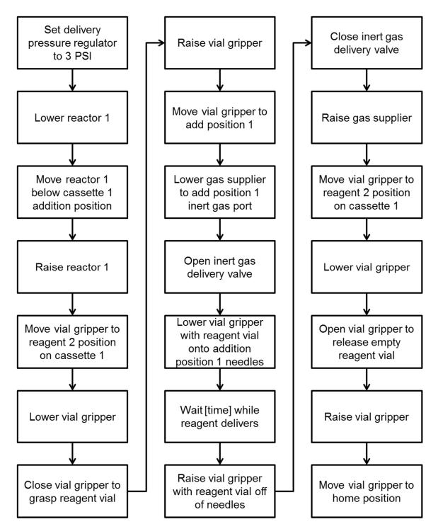
Supplementary Figure 1. Flowchart of 'Add' unit operation. Sequence of low level steps required to add the contents of a reagent placed in the second reagent position of the first cassette to the first reaction vessel. The user need only choose the 'Add' unit operation and set a few parameters; the low level details are carried out automatically.
