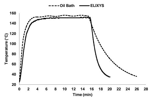
Supplementary Figure 2. Internal temperature of liquid in the reaction vessel during heating and cooling in the ELIXYS system and in an oil bath.
