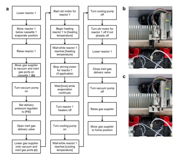
Supplementary Figure 3. (a) Sequence of low level steps required to evaporate the contents of the first reaction vessel. (b) Gas supplier is positioned over the vacuum and inert gas ports of the cassette. (c) Gas supplier is lowered, supplying vacuum and inert gas to the reaction vessel.
