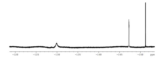
Zoomed out view of NaBF<sub>4</sub> (4 mg/mL) after being heated in HCl (1 M) showing SiF<sub>6</sub><sup>2</sup> resulting from glass etching following F<sup>-</sup> release ( $\delta$  -131 ppm, broad singlet), proposed BF<sub>3</sub>OH<sup>-</sup> ( $\delta$  -147.5 ppm, quartet) and BF<sub>4</sub><sup>-</sup> ( $\delta$ -151.52, septet) and <sup>11</sup>BF<sub>4</sub><sup>-</sup> ( $\delta$ -151.57, quartet)).
