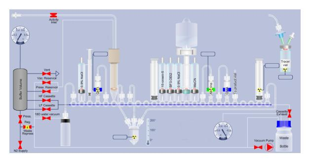
GE FASTlab<sup>TM</sup> cassette layout for [ $^{18}$ F]BF $_4$  $^-$  synthesis. SPE cartridges are conditioned as in the main manuscript. Reagents are present in cassette positions 2 (0.9% NaCl, 750  $\mu$ L), 12 (15-crown-5, 46 mg in MeCN (800  $\mu$ L)), 13 (BF $_3$ .OEt $_2$ , 0.2  $\mu$ L in MeCN (850  $\mu$ L)), 14 (0.9% NaCl, 1 mL), 15 (H $_2$ O (sterile purified water, GE Healthcare)) and 16 (MeCN, 1.5 mL).
