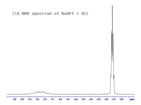
Expanded view of <sup>11</sup>B NMR spectrum of NaBF<sub>4</sub> (4 mg/mL) after being heated in HCl (1 M). Peaks correspond to BF<sub>4</sub><sup>-</sup> ( $\delta$  -0.7 ppm, quintet, J = 1.3 Hz) and suspected BF<sub>3</sub>OH<sup>-</sup> ( $\delta$  -0.2 ppm, quartet, J = 8.5 Hz).
