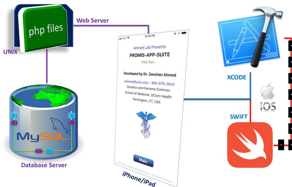
Figure S1. PAS-Gen components design, development, and data flow.
