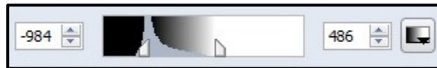
Figure 2 – Level (grey value) histogram after adjustment. Notice how the left slider is at the highest grey value peak and the right slider is at the maximum grey value present
